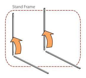
**27** B x1 BRD082 R x2 Ensure that wood board **(B)** is inserted first followed by a plastic spacer **(R)** on each side. Ensure that they are slid to the bottom of the channel.
